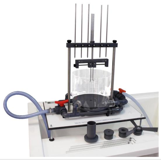
The objective of this team is the visualization and study of the formation of free and forced vortices. Is called **Forced Vortex** to the rotation of a fluid that moves like a solid with respect to an axis. By definition, in the forced vortex each fluid particle has the same angular velocity.
